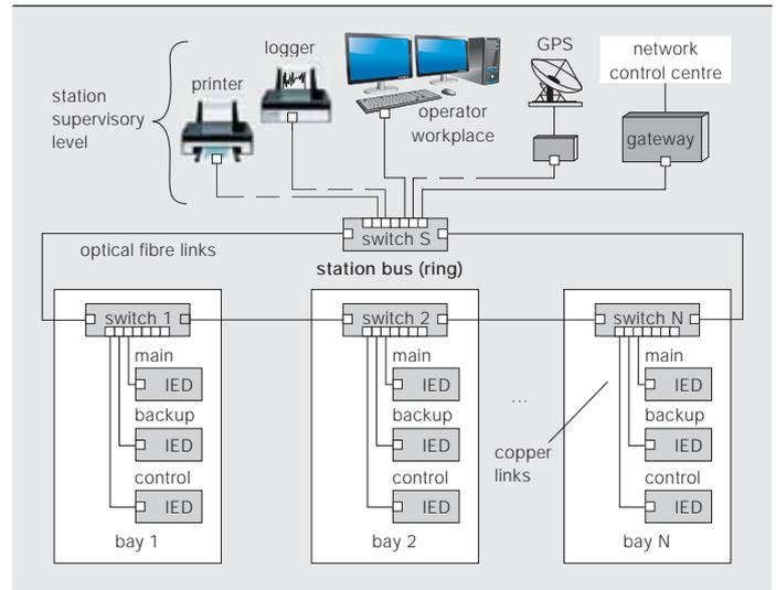
all transmitted information and provide zero-switchover time if links or switches fail, thus fulfilling all the difficult real-time requirements of substation automation.
