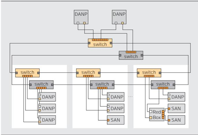
– Redundancy in the nodes. A node is attached to two different redundant networks of arbitrary topology by two ports → 5. Each node independently chooses the network to use. This scheme supports any network topology; the redundant networks can even exhibit a different structure. The cost of implementing this redundancy method is about twice that of the redundancy method discussed in the previous bullet, but the gain in availability is large. The only non-redundant parts are the nodes themselves.
