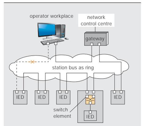
physical Ethernet network could carry both the station and the process bus traffic.
