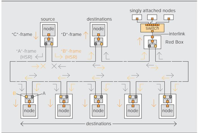
ring and every node forwards the frames it receives from one port to the other. When the originating node receives a frame it sent itself, it discards it to avoid loops; therefore, no special ring protocol is needed.
