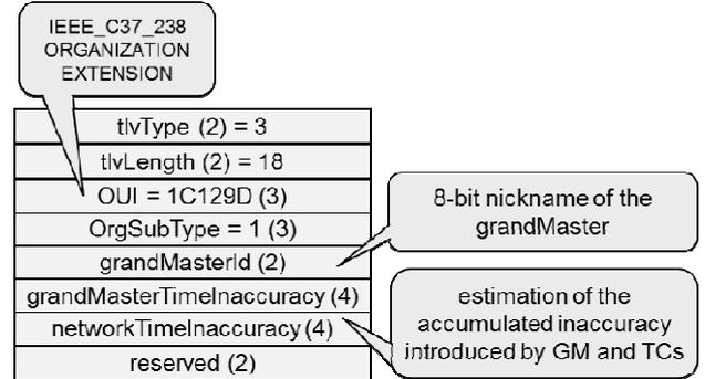
Figure 1. C37.238-specific TLV (tivLength corrected).
